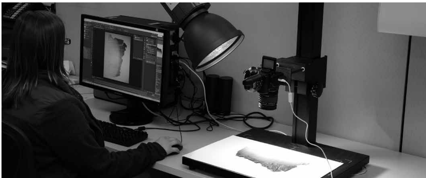
Preservation technician Meghan Krato uses an infrared camera and computer software to recover lost information on a burned record.
